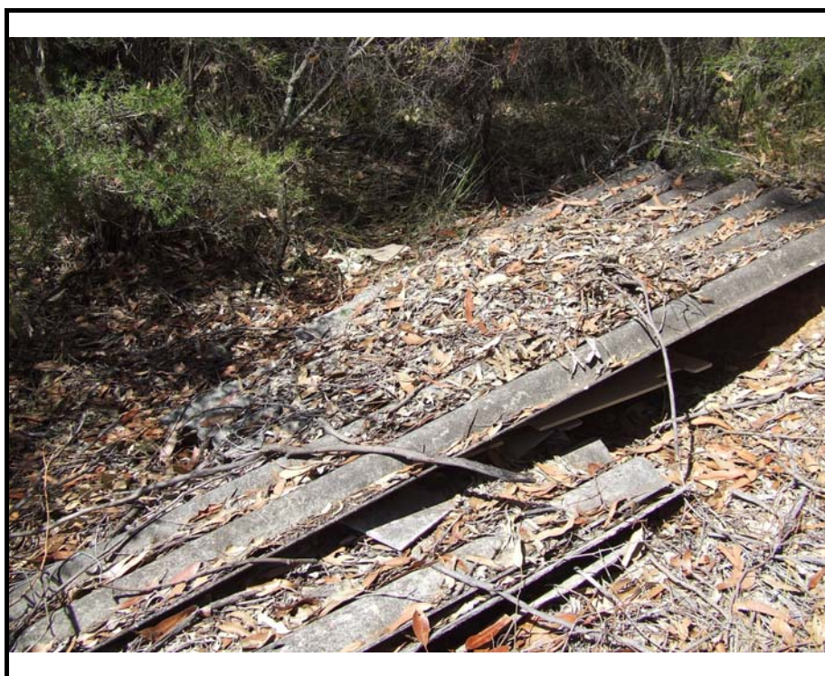
Photo 2: Photograph of dumped Super Six sheeting (asbestos containing material) in the northern portion of Employment Land Parcel 7.
